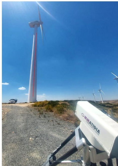
Figure 3: deployment of Q1 LDV in the field. The dotted line is superimposed to show the measuring points
