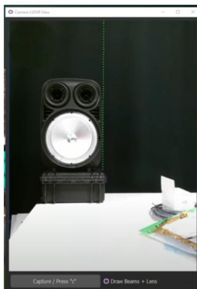
Figure 2: left: field view from Q2. The green dotted line represents the 65 measuring points. Right: by scanning the azimuthal angle, the full-field view measurement is obtained
